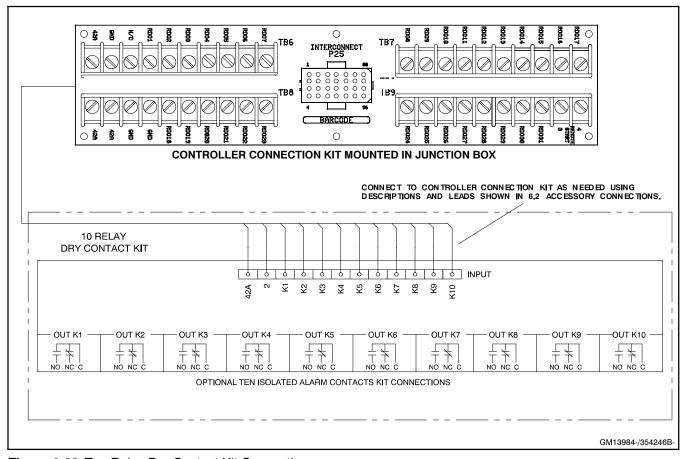
Figure 6-33 Ten-Relay Dry Contact Kit Connections
